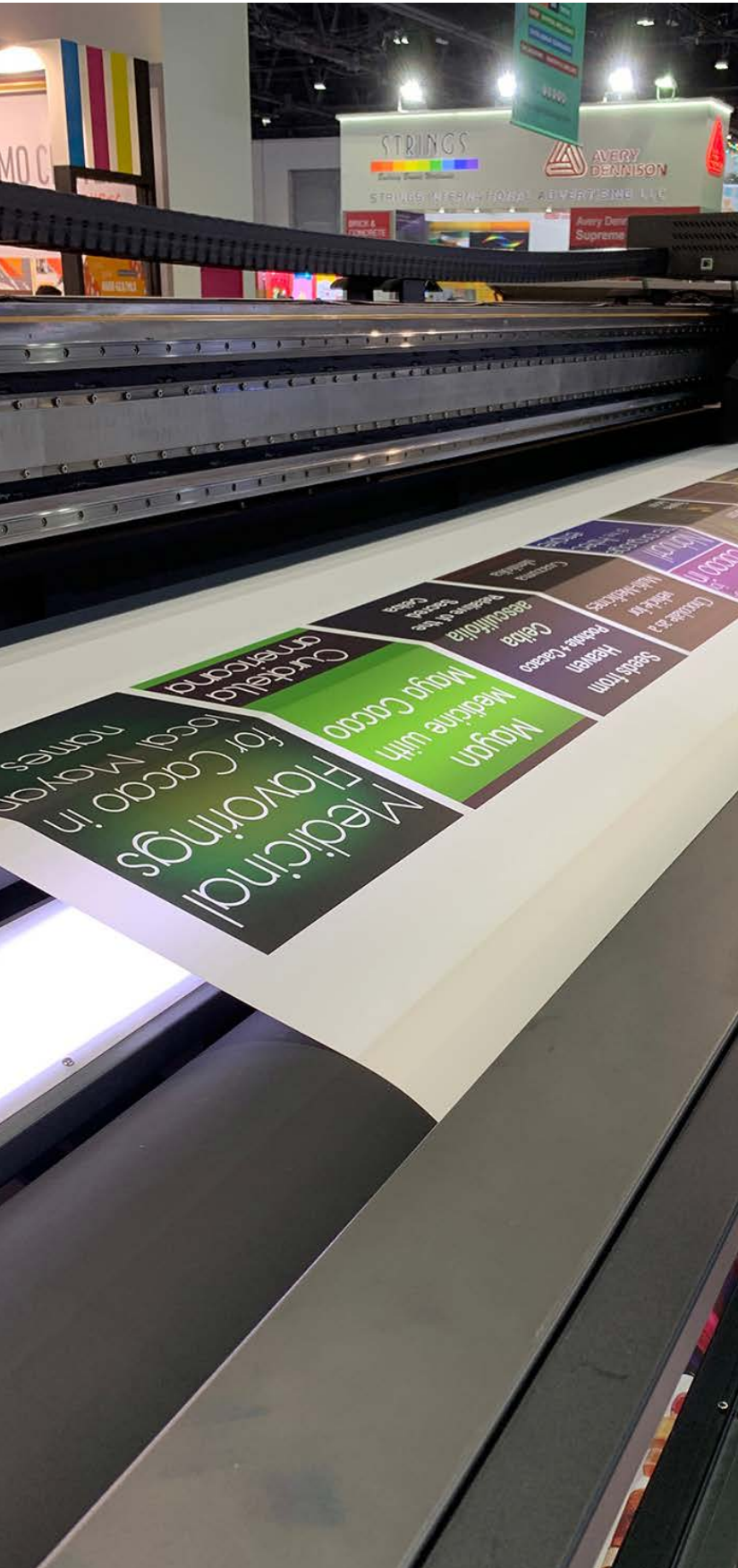
Test prints are a good way to be able to see print quality. So here we are testing a UV-curing printer from Plamac.
